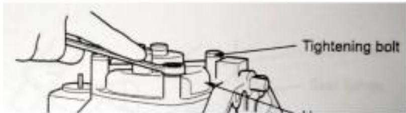
Figure 3: Step 1: Remove Upper Gear Tightening Bolts (4) And Upper Gear Cover
