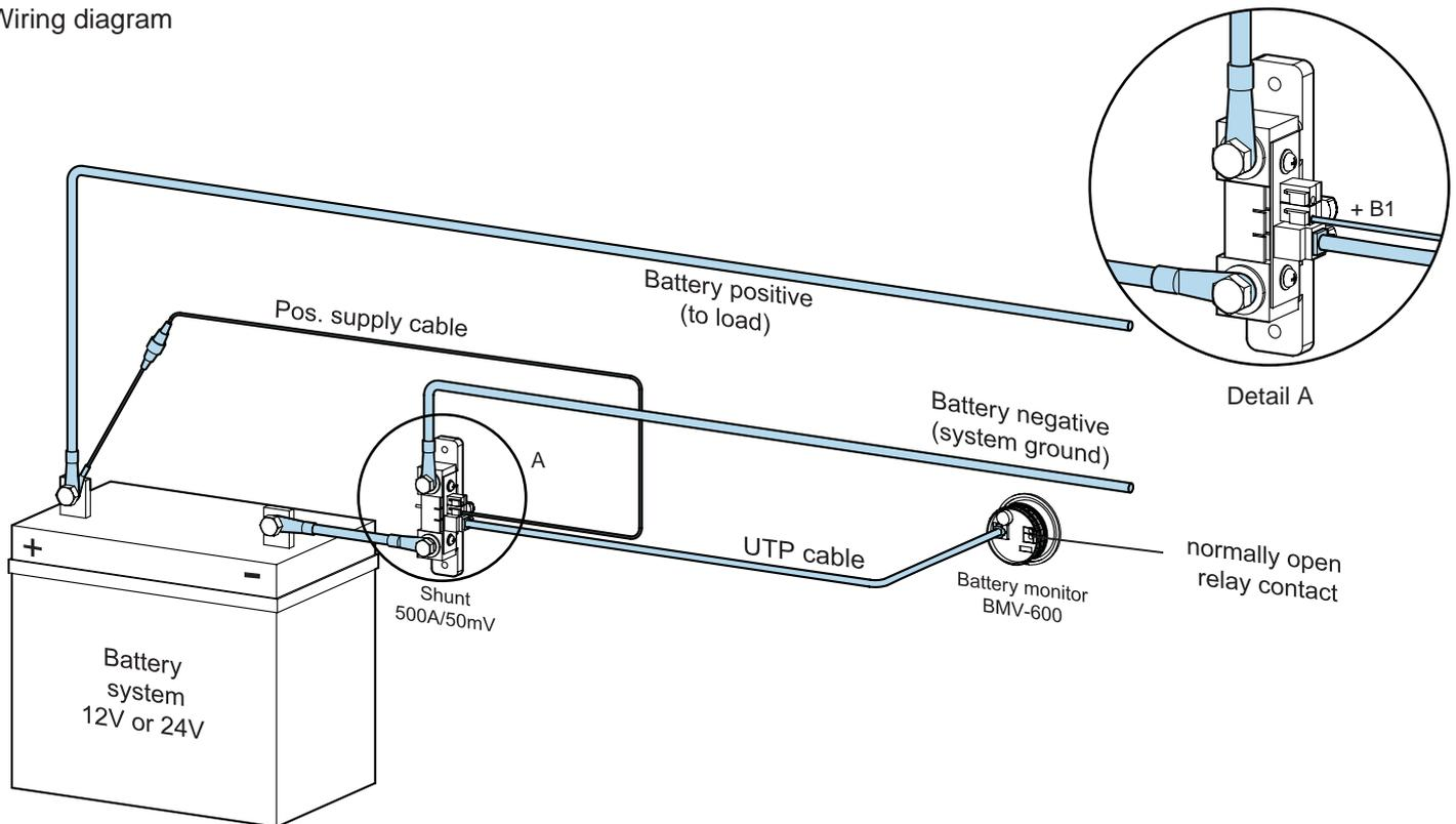
**Connect the negative pole of the battery last !**
