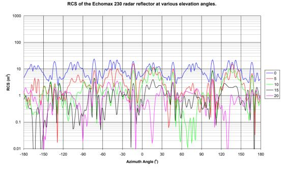
Figure 18 RCS of the Echomax 230 radar reflector.
