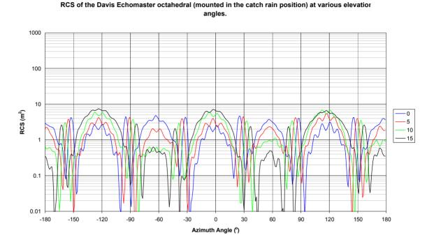
Figure 15 Plot of linear RCS of the Davis Echomaster octahedral radar reflector.
