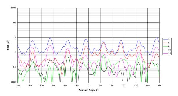
Figure 14 Plot of linear RCS of the Plastimo 4" Tube.
