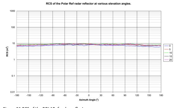
Figure 21 RCS of the POLARef radar reflector.
