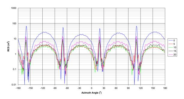
Figure 12 Plot of linear RCS of the Plastimo 16" Octahedral reflector when mounted in the upright position.
