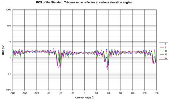
Figure 17 RCS of the Standard Tri-Lens radar reflector.
