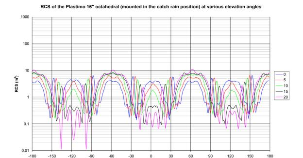
Figure 13 Plot of linear RCS of the Plastimo 16" Octahedral reflector when mounted in the catch rain position.
