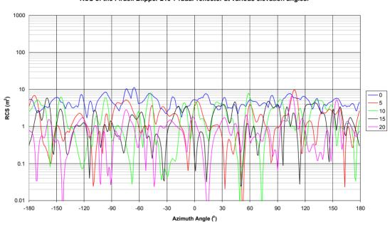
RCS of the Firdell Blipper 210-7 radar reflector at various elevation angles.
