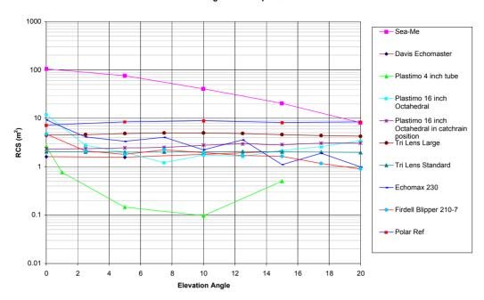
Figure 23 Comparison of each of the radar reflector's average RCS.
