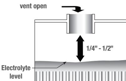
Figure 8 – Electrolyte level
