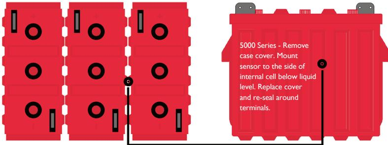
Figure 7 – Temperature Probe
