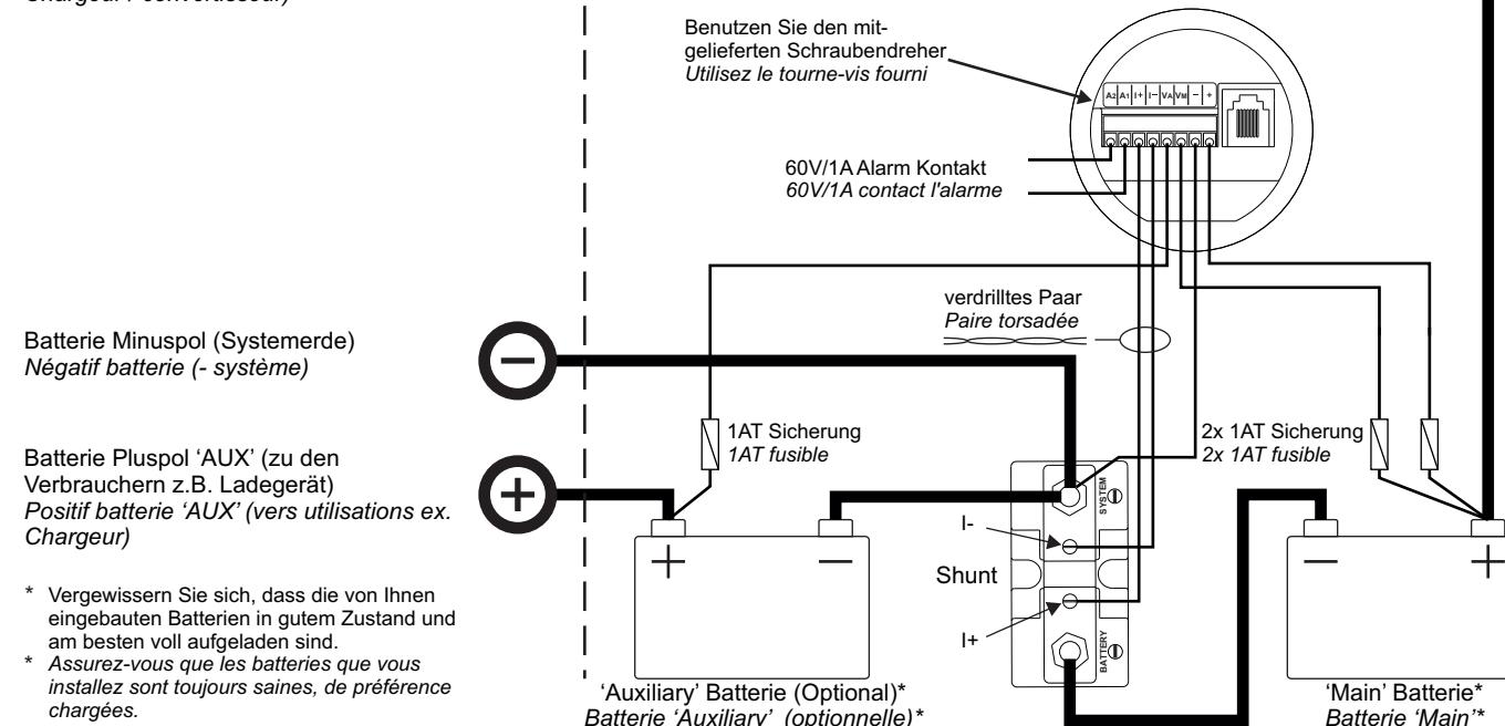
**WARNING** The shunt must always be installed into the negative line!
