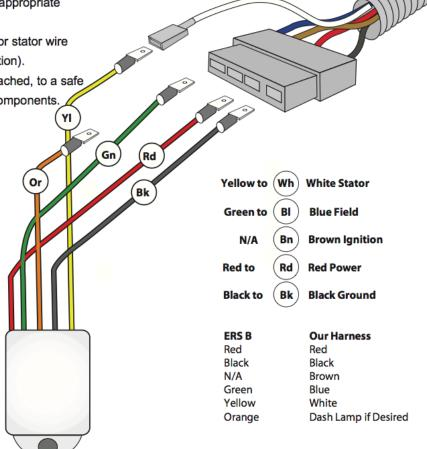
In addition to it's use with the standard Balmar wiring harness, the ERS regulator can be used in conjunction with any 12-volt P-Type alternator. The ERS Regulator Kit includes the following terminal connectors, which can be used to modify the ERS wiring to suit your specific application (see sample installation diagram on other side of instruction sheet):
