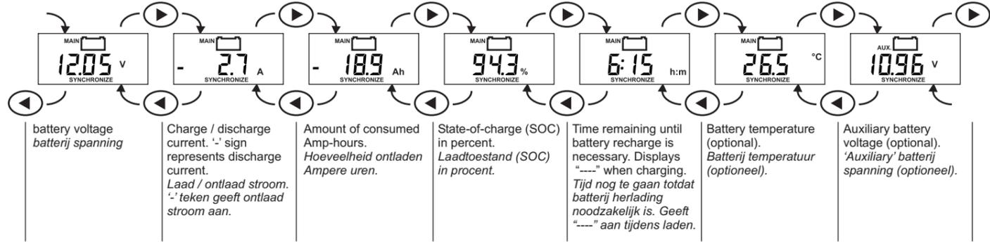
The display also indicates *SYNCHRONIZE*. As will be further explained in the owner's manual, this message means that the battery needs to be fully charged first, in order to synchronize the battery monitor with the battery. Otherwise, the State-of-charge readout will be invalid. The more often you are fully charging your batteries, the more precise the battery monitor will indicate all parameters. This will also result in a longer lifetime of your batteries.
